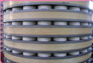
Iron Core Divided by Air Gaps
